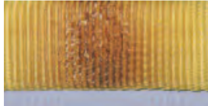
Melting or charring of the tiedown, or weld splatter on the tiedown
