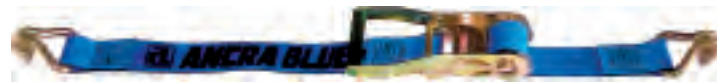
45982-85-27 2-in. x 27-ft. ANCRA BLUE Ratchet Strap w/ 43120-13 Wire Hooks. Fixed End 18".
