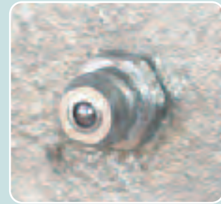
Grease fitting simplifies routine maintenance
