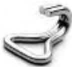
40316-12 1-inch Narrow Hook. WLL: 166 lbs./75 kg. Weight: .10 lb./05 kg.
