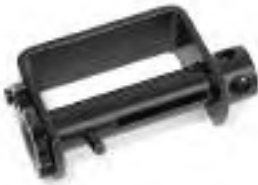
41681-10 Standard Bottom Mount Weight: 10.6 lbs./4.8 kg. WLL: 5,500 lbs.
